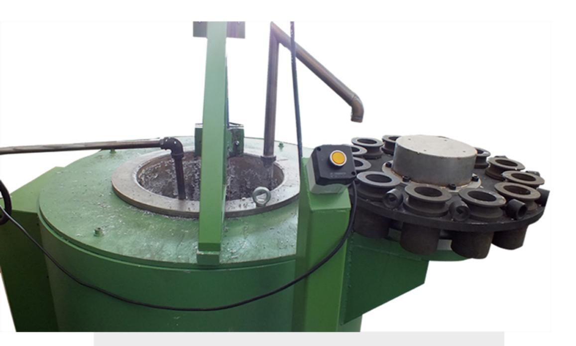
Leadmac's lead block melting and casting machine is able to produce lead blocks with any dimensions of shapes.
